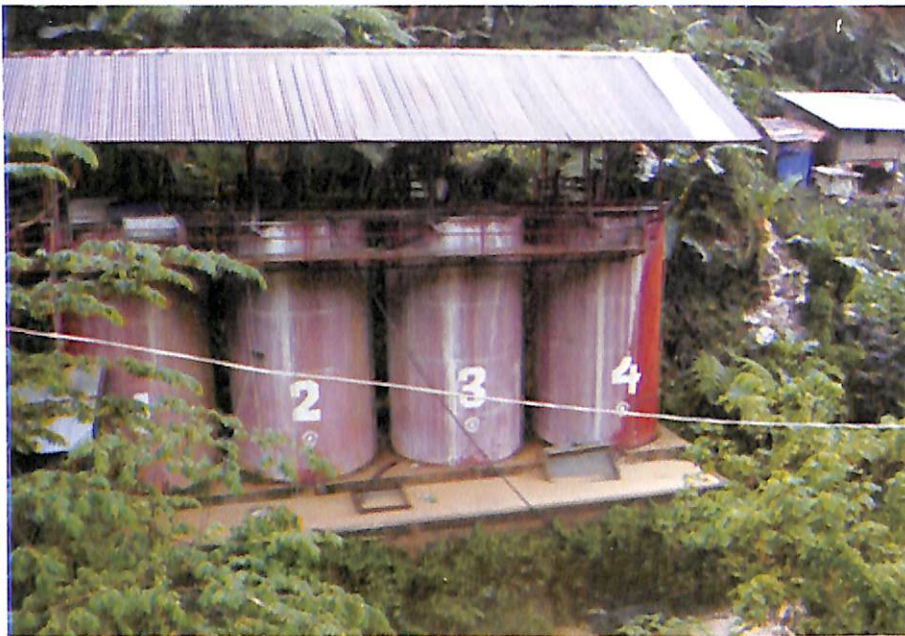
Figure 4: A Carbon-In-Pulp (CIP) planta somewhere in Compostela Valley Photo courtesy of Adrian Daniel
